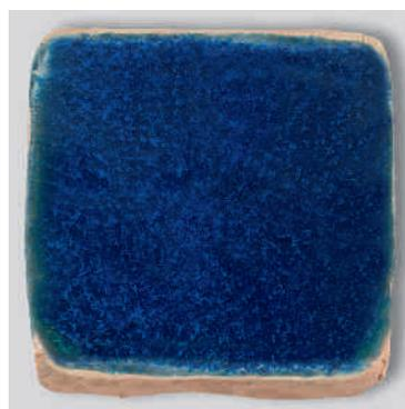
*The glaze made from the heated and quenched ingredients with 2% copper oxide and 0.1% cobalt oxide after the cuneiform recipe, applied with gum arabic to a raw, lime-rich body fired to 1030°C and soaked for 1 hour. The differing circumstances that stem from using an electric kiln and pure ingredients have been taken into consideration as far as possible. In such archaeological experiments, there is no guarantee that the actual processes from the past have been reproduced.*
